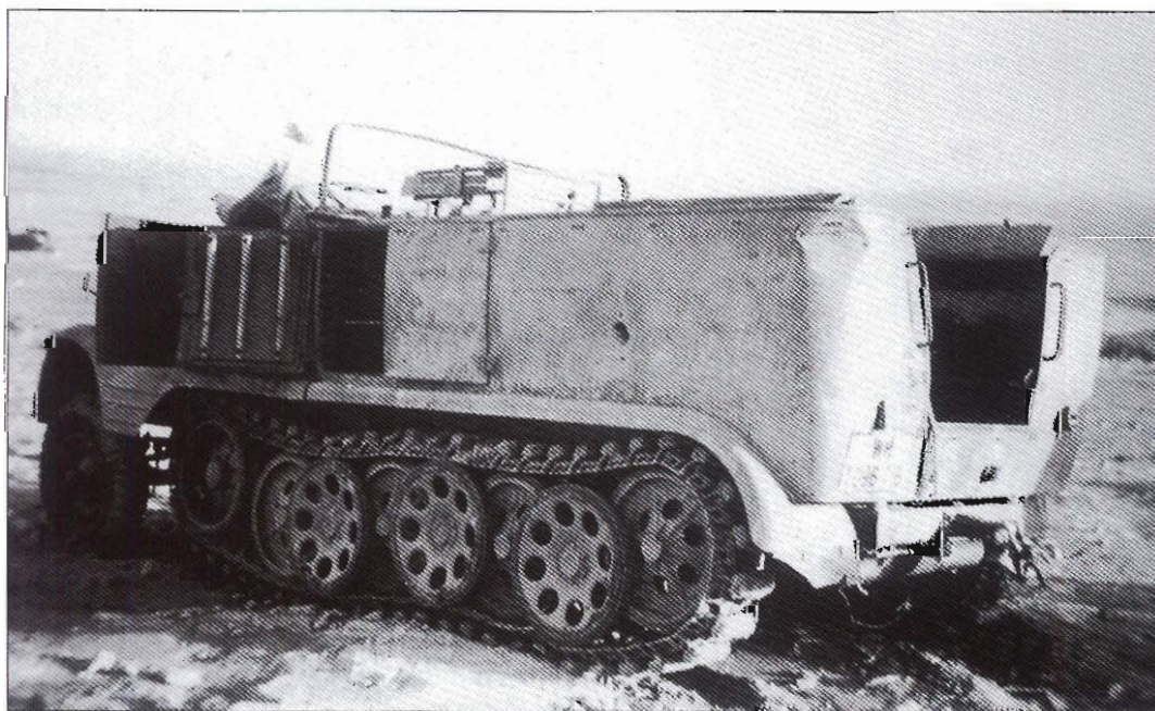
A derelict Sd.Kfz. 11 half-track prime mover abandoned in the desert. These vehicles were mainly used to tow the 10.5cm leFH 18 howitzer in addition to other types of anti-tank and field artillery. The only visible marking is the Wehrmacht registration number painted on the rear.
