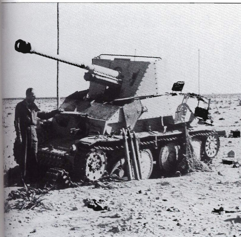
Two photos of a Marder III disabled by a mine blast that has blown off one of the roadwheels and broken the track. These vehicles were armed with captured Russian 76.2mm M1936 field gun, designated FK296 by the Germans, the same gun that was installed on the 'Diana'. It was redesigned and numbered to take the German PaK 40 ammunition. Markings are limited to a black and white national cross painted on the sides and on the smoke gas cover on the rear of the vehicle.
