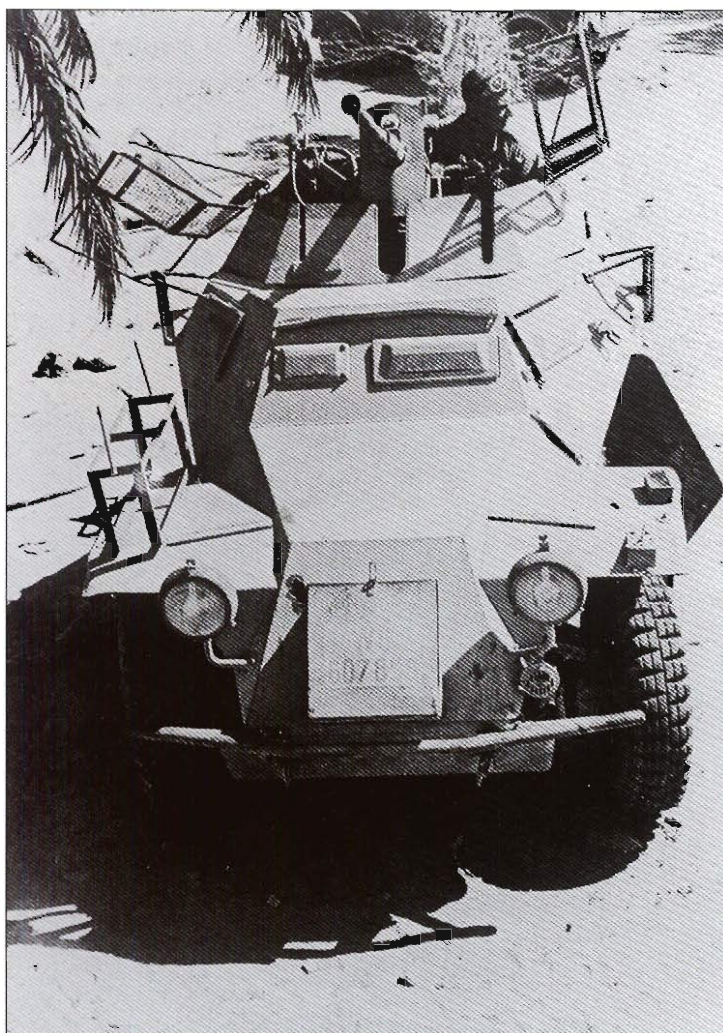
British soldiers inspect another Sd.Kfz. 222 that looks relatively intact however note the penetration hole in the front plate next to the storage box. It is similarly marked to the other vehicle but the remnants of a tactical marking appear on the left side engine compartment access door. The vehicle registration number - WH 607858 - is painted on the front and rear and a faint 15. Panzer-Division emblem can be seen on the left mudguard between the Nottel light base and headlight.
