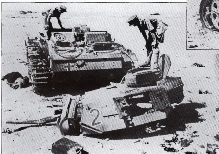
This Pz.Kpfw III Ausf J of 2 Kompanie/Pz.Rgt.8 was destroyed near Tobruk in June 1942. The tactical number '2' is painted in a white outline on each side of the turret. The national cross is also painted in white. While the Pz.Kpfw III Ausf.J was more than capable when dealing with the Crusader and Stuart tanks, it was less powerful than the newly introduced Grant.
