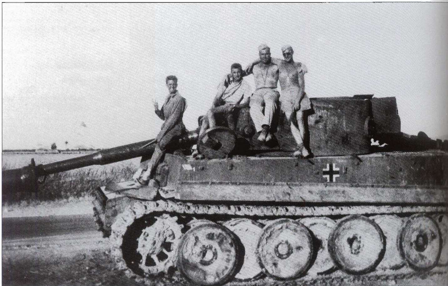
A Pz.Kpfw VI Ausf E 'Tiger I' of 1 Kompanie/s.Pz.Abt.504 knocked out near Tunis by British forces. The small white rhombus with a '1' beside it can be seen on the front side of the hull along with a white outline black national cross midway down the side. An internal explosion has blown off the commander's cupola and barrel sleeve, pushing it down against the muzzle brake. Note the Feifel air cleaners just visible on the rear of the vehicle.
