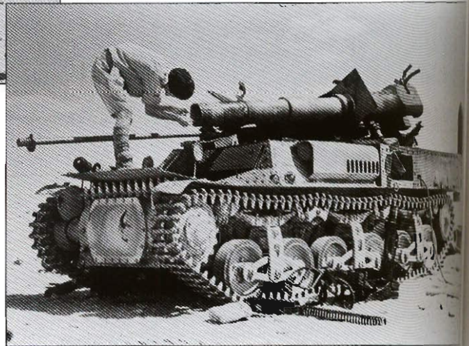
A 15cm sFH 13 (Sfl.) auf Lorraine-Schlepper from Pz.Art.Rgt 155, 21 Panzer-Division, destroyed at El Alamein in September 1942. Twenty-three of these self-propelled howitzers were shipped to North Africa in July and August 1942, ten to Pz.Art.Rgt 155 and thirteen to Pz Art.Rgt.33 of 15.Panzer-Division. All were reported to have been destroyed by December 2 1942
