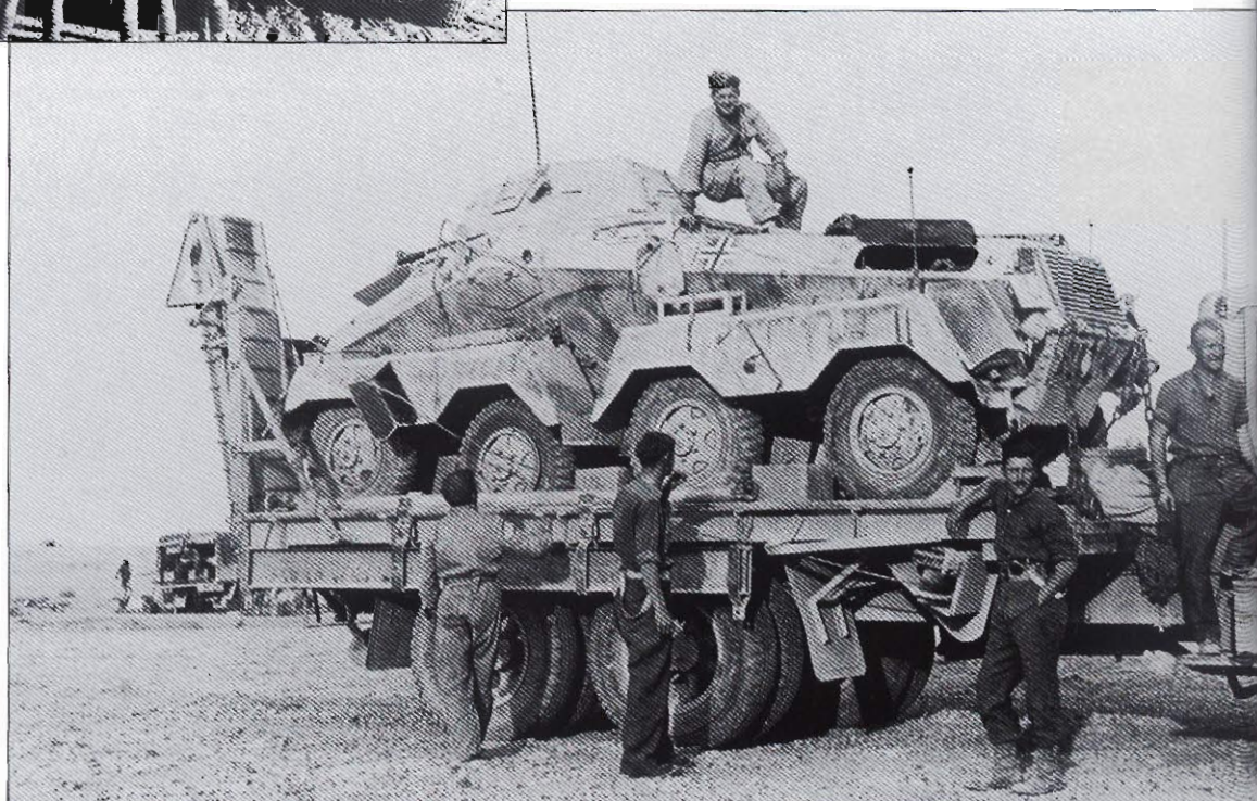
A schwere Panzerspähwagen Sd.Kfz.231 loaded onto a British transport truck for removal. The vehicle is possibly for further evaluation. The yellow camouflage paint is well shown, as is the dark base underneath. Markings are limited to the vehicle registration number plate and the original white outline national cross. A Panzer appears the half-repeated the trailer visible a DAK pair the red emblem. Two stor been on the road way.
