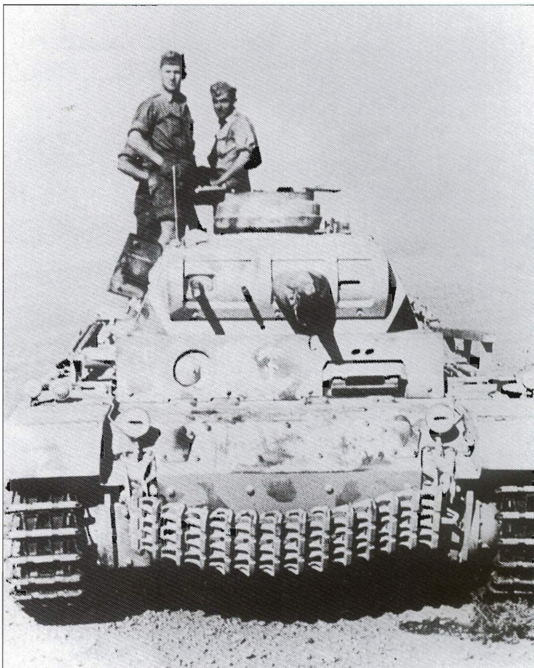
The crew of this Pz.Bef.Wg.III Ausf.H pose with the r war booty - some captured bottles of wine. The turret was bolted in place and the large frame antenna on the engine deck distinguished this tank from the standard gun tank. Later in the war, it was replaced by the less conspicuous star antenna. Two crew members wear the tropical sun helmet which, though unpopular, continued to be worn until the end of the campaign
