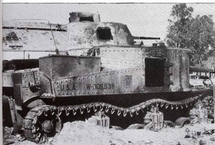
An American M3 Lee knocked out near Sened, Tunisia in March 1943. The serial number is painted in blue on the olive drab base color and a name, possibly 'San Juan' is painted in white just behind the 75mm gun mount. The resulting fire has burned off the paint on the side of the hull and 37mm gun turret, leaving the outline of the yellow or white star painted on the side of the turret faintly visible. The armor of the M3 was no match for the guns of the Pz.Kpfw IV Ausf. F2 or G and Tiger I.
