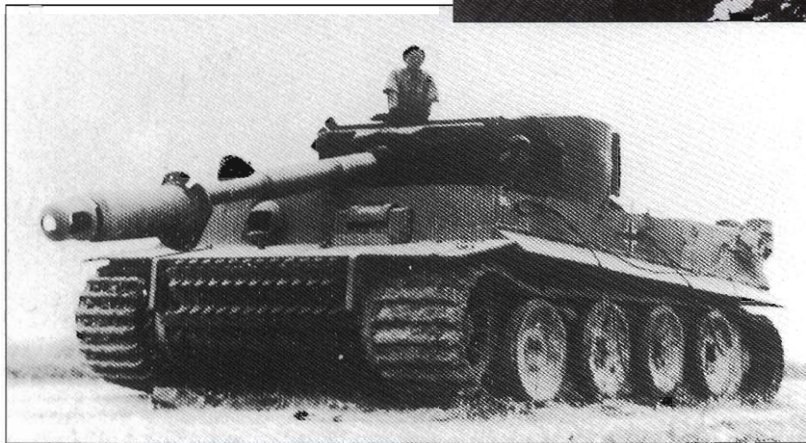
A Pz.Kpfw VI Ausf E 'Tiger I' of 1 Kompanie/s.Pz.Abt.504 knocked out near Tunis by British forces. The small white rhombus with a '1' beside it can be seen on the front side of the hull along with a white outline black national cross midway down the side. An internal explosion has blown off the commander's cupola and barrel sleeve, pushing it down against the muzzle brake. Note the Feifel air cleaners just visible on the rear of the vehicle.
