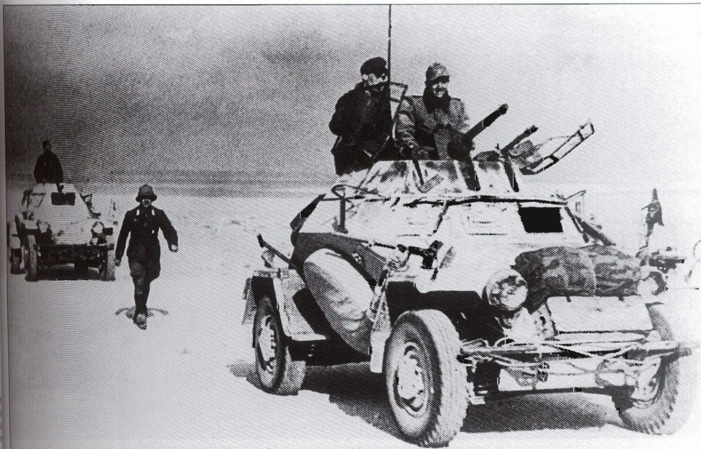
An early production leichte Panzerspähwagen Sd.Kfz.222, armed with a 2cm KwK30 and a coaxial 7.92mm MG34, is followed by an Sd.Kfz.221 which was armed only with an MG34. The Sd.Kfz.222 shows a well worn paint scheme of desert sand paint applied over the dark gray base. No markings are visible on either vehicle.
