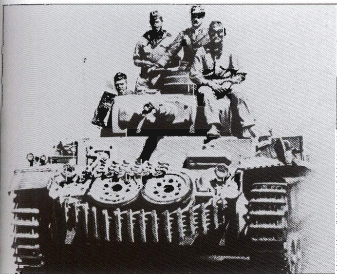
An early Pz.Kpfw.III Ausf. G of Pz.Rgt.5 raises a cloud of dust as it travels down a desert road. The additional roadwheels and spare track also served to provide additional protection for the vehicle. It has been painted with a light coat of sand yellow applied over the dark gray base color. The object visible to the left of the turret is a telegraph pole.
