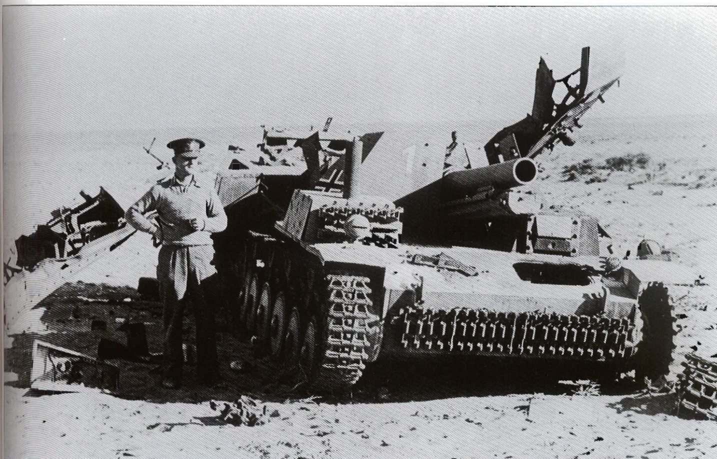
A 15cm s.I.G.33 B SII from s.I.G.Kp (mot S) 707 or 708 that has been destroyed by an anti-tank round that has set off the ammunition stored in the back of the vehicle. Twelve of these self-propelled guns were sent to Libya, six in February 1942 and the remainder in April. The weight of the gun overloaded the chassis and they suffered from many automotive problems during their short combat history. After the battle of El Alamein, the British reported capturing six in various states of repair. German reports indicate that all were lost by December 2, 1942.
