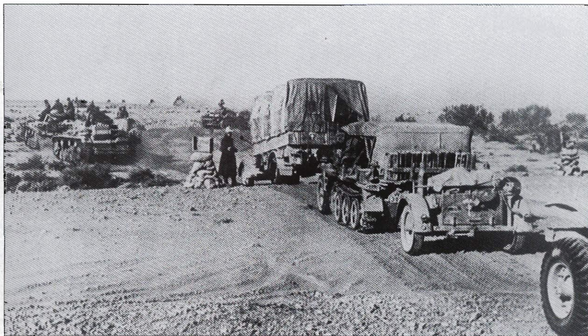
An Sd.Kfz. 7 half-track towing a 15cm sFH 18 howitzer into a prepared emplacement in January 1942. The sand yellow camouflage paint is almost worn off the half-track exposing the dark gray base while the gun shows wear mostly around the gun barrel. A small enclosure has been set up using some wooden crates and the wicker shipping containers that the 15cm projectiles were shipped in. The tactical sign for a towed artillery company can be seen on the left mudguard of the Sd.Kfz. 7
