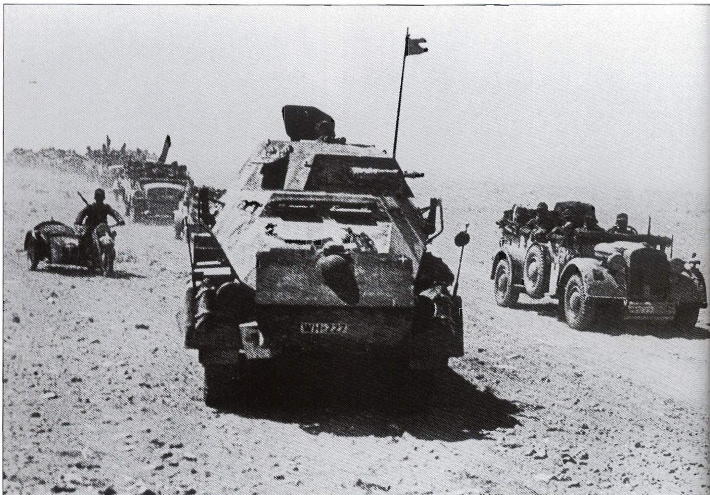
A column of light transport vehicles is led by an early production schwere Panzerspähwagen Sd.Kfz.231 eight wheeled armored car fitted with additional 8mm armored shield which was added to the front beginning in early 1940. The Horch Kfz. 15 on the right displays a DAK palm emblem on left mudguard and an unidentifiable tactical marking on the right on a patch of the original dark gray paint.
