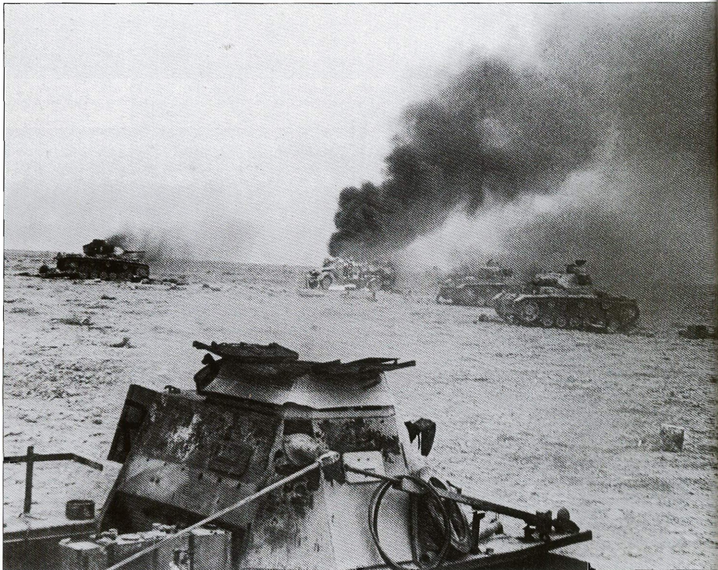
The remains of three Pz.Kpfw.III and a lorry from Pz.Rgt.8 burn in the background after an intense battle. The Pz.Kpfw.III on the right is an Ausf.H, the one beyond it is an Ausf.G. In the foreground is a Kfz.Pz.Bef.Wg.I Ausf.B that has had its rear engine deck blown off. Part of the tactical number, probably a black 'R', can be seen on the open hatch door.
