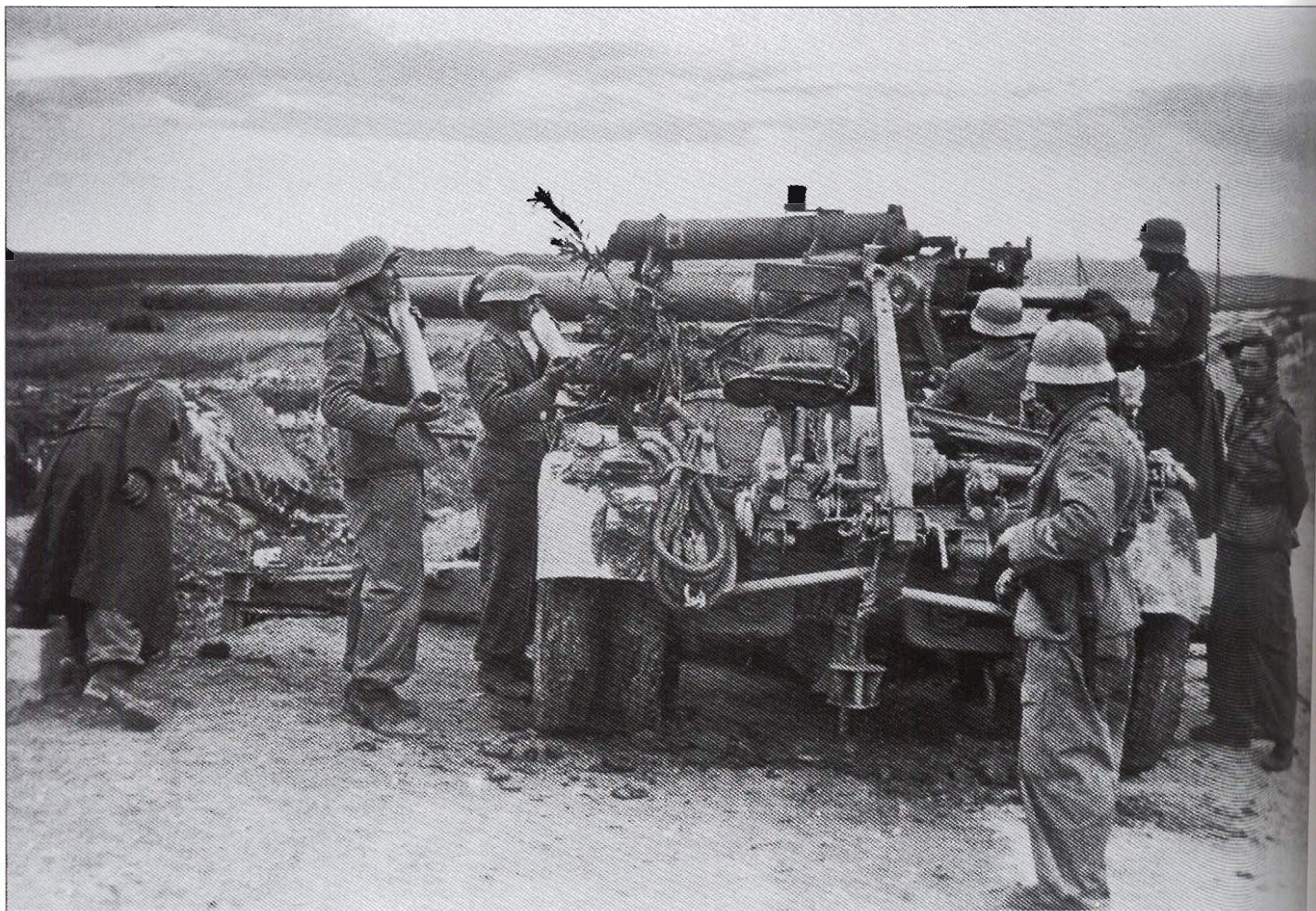
An 8cm FlaK 18 anti-aircraft gun of a Luftwaffe Flak-Regiment fires at ground targets near Tebourba in January 1943. The gun is carried on the newer Sd.Ah 202 trailer, equipped with four sets of dual tired wheels which is waiting close by in case the gun needs to be moved in a hurry. The crew seem to all be wearing the Luftwaffe tropical uniform with the large patch pocket on the left leg of the trousers. The crewman in the foreground has the Flakartilleriepersonal specialist badge on his left sleeve which was awarded after nine months service.
