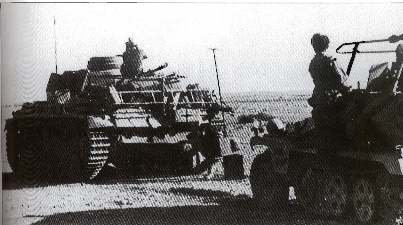
The commander of this Pz.Bef Wg.III Ausf H intently scans the horizon with his binoculars. In the foreground is Rommel's early Sd.Kfz.250/5 half-track, nicknamed 'GREIF', which is painted on the left side in red with a white outline and on the right side in white outline only. Just visible behind the tank is a radio operator seated at a field radio. The turret of the Pz.Bef Wg.III was fixed in place thus permitting the engine deck to be used for stowage of additional gear. This photo was taken on July 16, 1942
