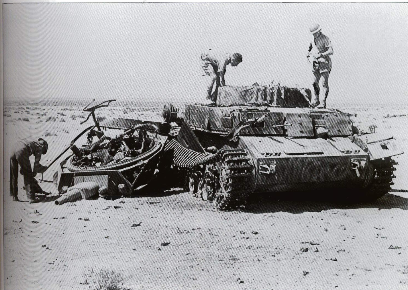
A Pz.Kpfw.IV Ausf.E of Pz Rgt.5 completely destroyed by an internal ammunition explosion that has blown off its turret. The 20mm and 30mm additional armor plates are quite visible in this photo. During the attack on Tobruk, 8 Kompanie lost 5 of its Pz.Kpfw IV. Sand yellow paint has been applied in a thin, wavy pattern over the dark gray base. The object in front of the driver's visor is one of the return roller mounts from the side of the vehicle. This vehicle is still fitted with the early 36cm track.
