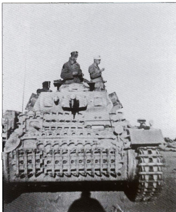
This Pz.Kpfw.III Ausf. H is identified by the additional 30mm armor plates bolted on the front of the hull and welded to the front of the superstructure. The crew has added several sets of extra spare track links to further increase the protection.
