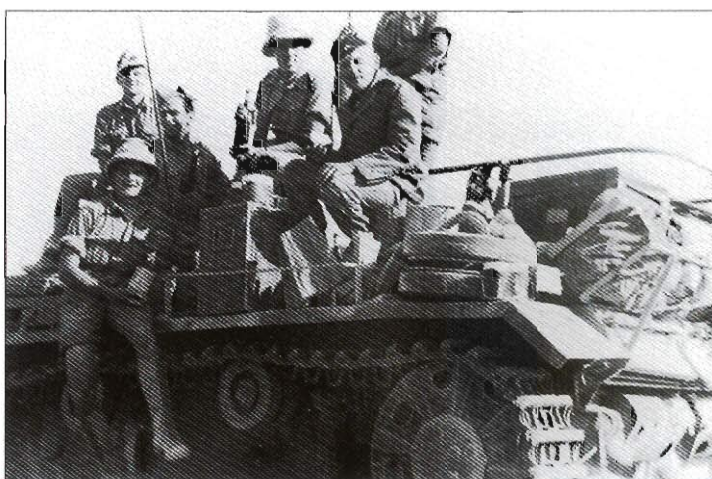
The crew of this Pz.Bef.Wg.III Ausf.H pose with the r war booty - some captured bottles of wine. The turret was bolted in place and the large frame antenna on the engine deck distinguished this tank from the standard gun tank. Later in the war, it was replaced by the less conspicuous star antenna. Two crew members wear the tropical sun helmet which, though unpopular, continued to be worn until the end of the campaign
