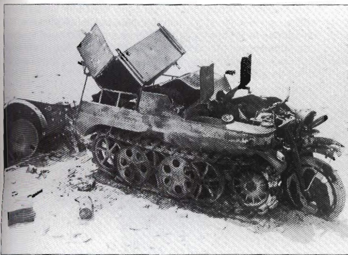
Another Kettenkrad destroyed when small arms fire ignited the fuel from its gas tanks causing the vehicle to burn. It is towing the standard trailer built especially for use with the Kettenkrad. The remains of a Divisional Services tactical marking, a rectangle with an 'X' inside, can be seen on the side of the engine compartment.
